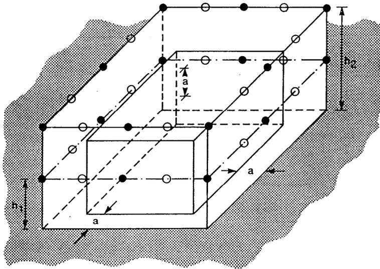
Fig 7 Example. illustration of key and additional microphone positions.
