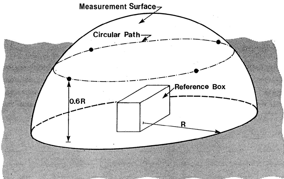
Fig. 4 Circular path on hemispherical measurement surface.
