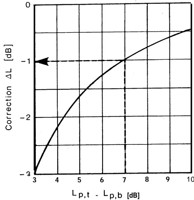
Fig B.1 Diagram for determining the correction L for background noise, see text.
