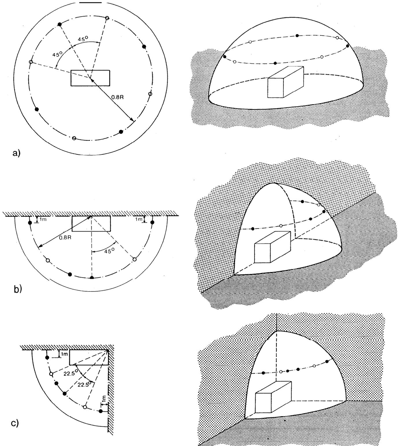
Fig 5 Spherical measurement surfaces and microphone positions around a reference box
