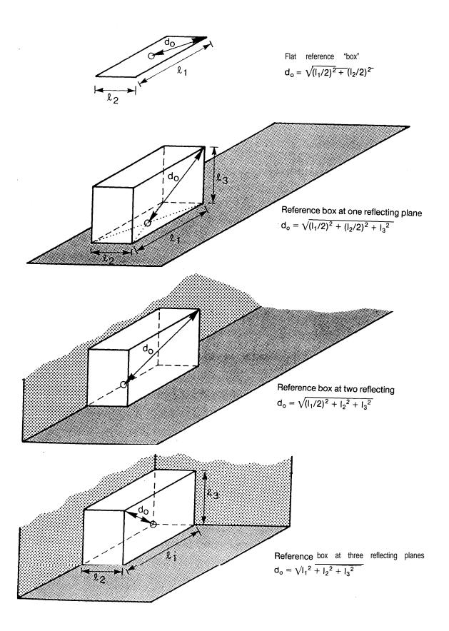
Fig. 2 Examples illustrating reference box and characteristic source dimension, d
