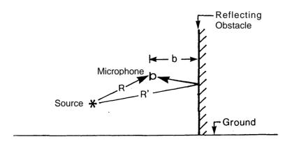
Fig. 3 Illustration of distances from source to microphone position.
