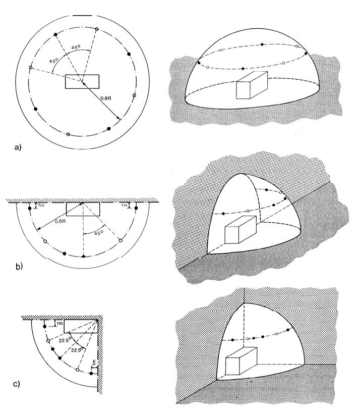
Fig 5 Spherical measurement surfaces and microphone positions around a reference box
