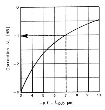
Fig B.I Diagram for determining the correction L for background noise, see text.
