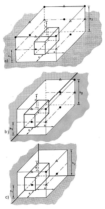
Fig 6 Measurement boxes terminating on a) one, b) two and c) three reflecting planes with key microphone positions.
